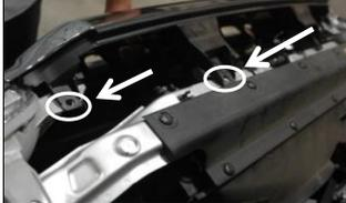
Remove 4 bolts located on top of the grill
