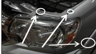
Remove 2 bolts located on top of the headlight and 1 bolt located
