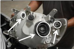
Once the headlight is out remove the turn signal harness, the parking lights harness and the low/high beam light harness
